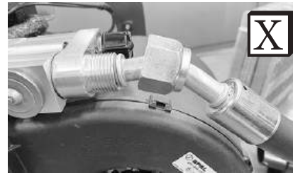
Improperly Seated O-ring Land
